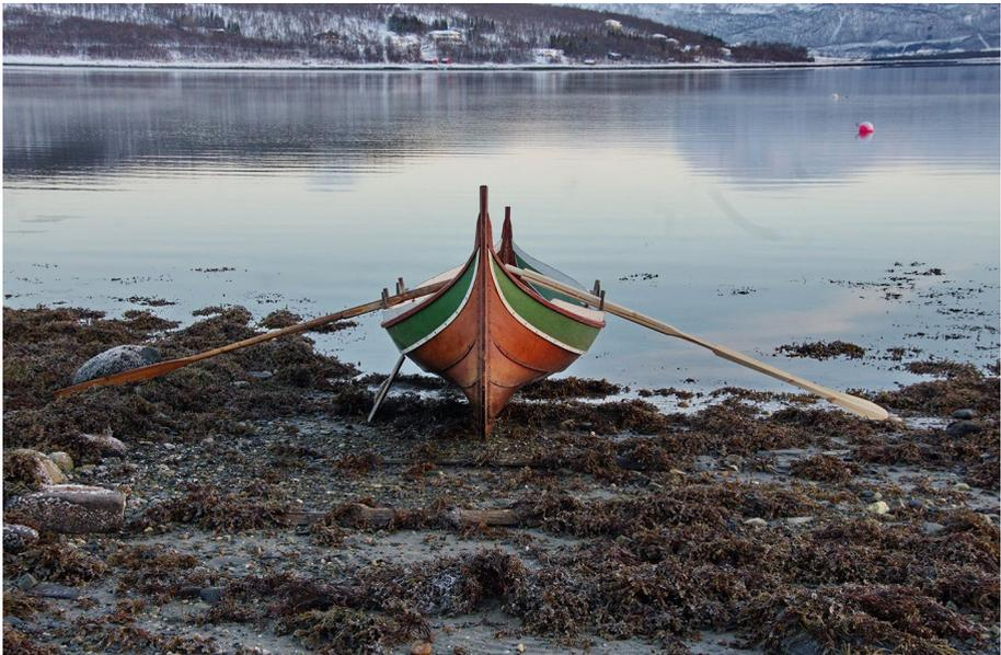
**Fig. 12** Photograph of Hersøy oar copy being used in a traditional northern Norwegian rowboat (*færing*). Gunnar Eldjarn, The Arctic University Museum of Norway
