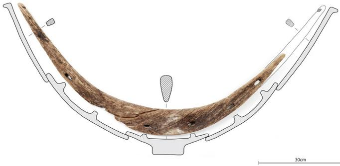
**Fig. 6** Boat frame from Grunnfarnes, Senja Island in Troms with suggested reconstruction. Adnan Içagic, The Arctic University Museum of Norway
